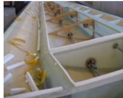
The glider is also constructed to distribute the forces and make them stronger. For example the wings have cross sections of wood and glass fiber to keep them from breaking (see right).
